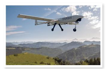
TARSIS-W is a NATO Class I UAS System with the capacity to integrate two 50 mm caliber micromissile launchers under each semi-wing, each launcher can house up to 2 semi-active laser-guided micro-missiles with a range of 4 km depending on the altitude of shooting. In addition, it includes an integrated Weapons Management System with the Ground Control Station to operate ammunition remotely and securely.
