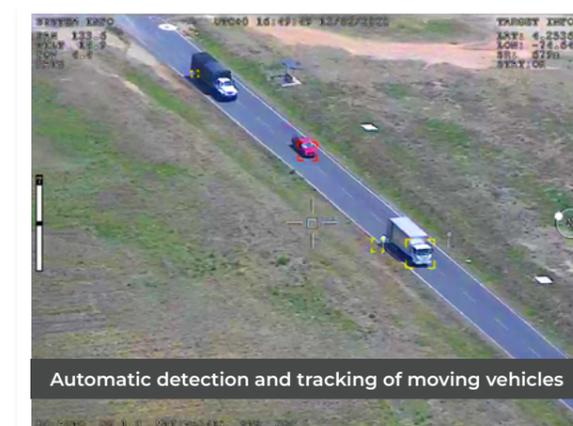
Automatic detection and tracking of moving vehicles
