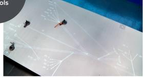
Projection of drawings on a 1:1 scale
