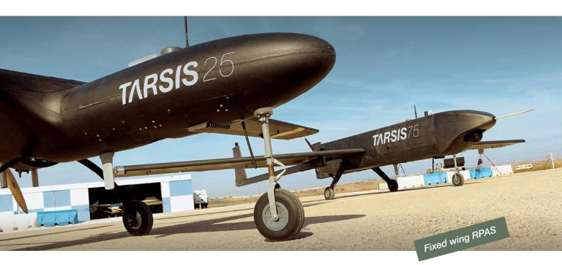
AERTEC Solutions has developed a complete family of RPAS (Remotely Piloted Aerial Systems). The TARSIS aerial platforms stand out among most fixed-wing unmanned aerial vehicles of similar size. The TARSIS family of RPAS are versatile fixed wing solutions capable of performing different missions with a variety of configurations mainly designed for observation and surveillance. AERTEC Solutions has currently two operative solutions:
